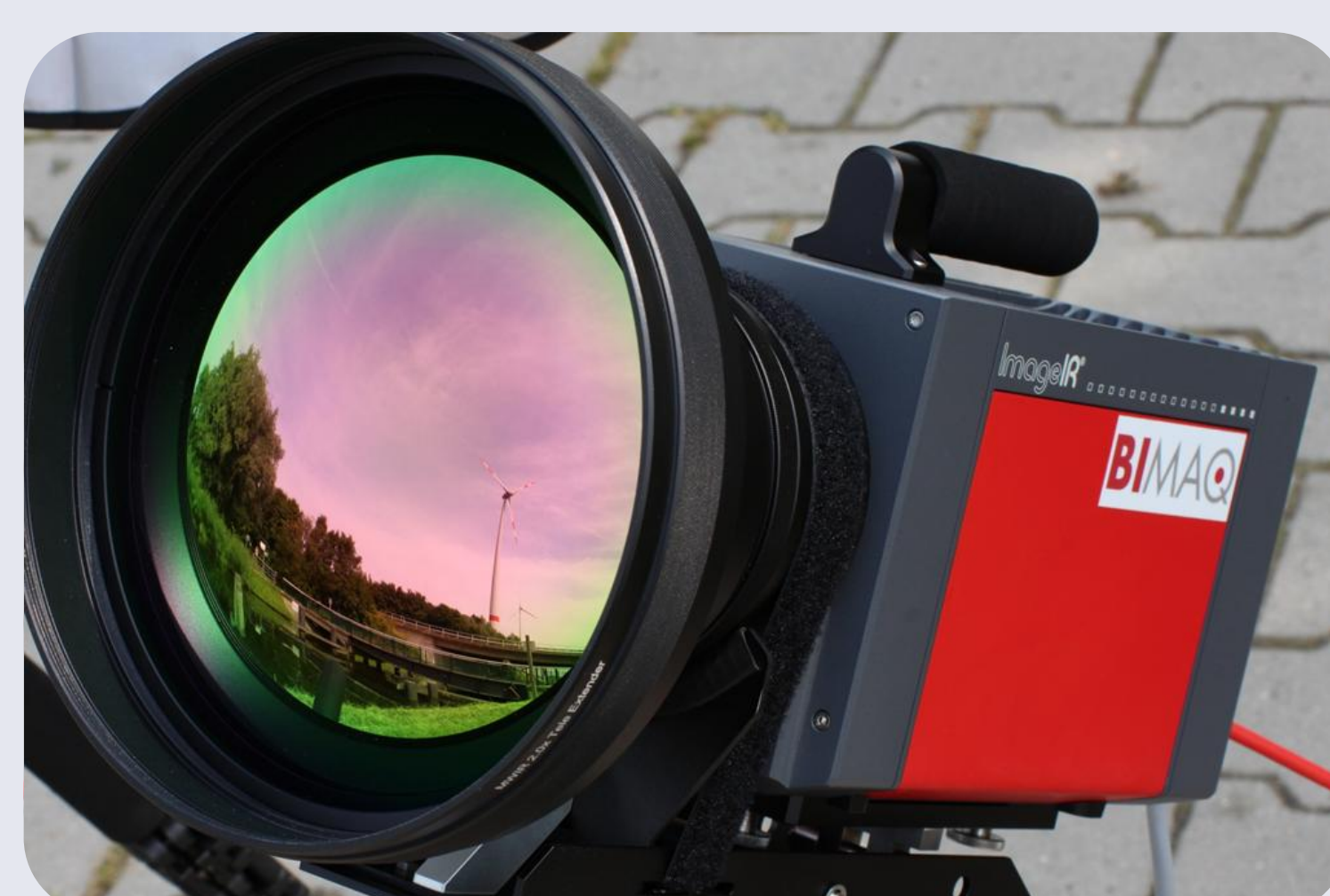
Fig. 5: Thermographic imaging system with telephoto lens.
